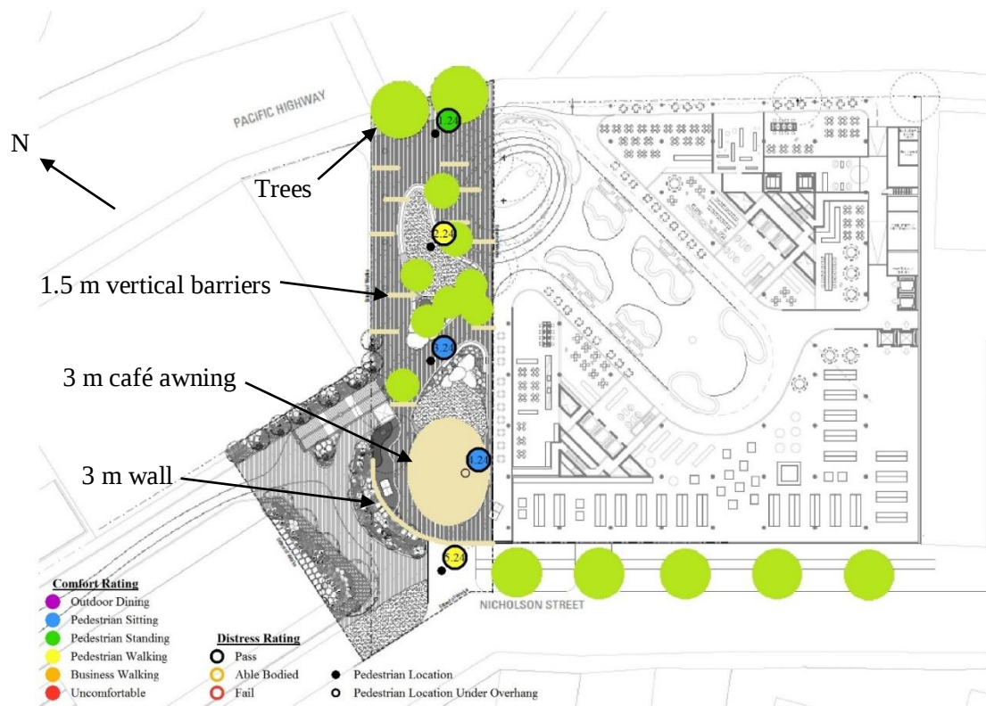
Figure 14: Pedestrian wind speed measurements – Configuration 2E
