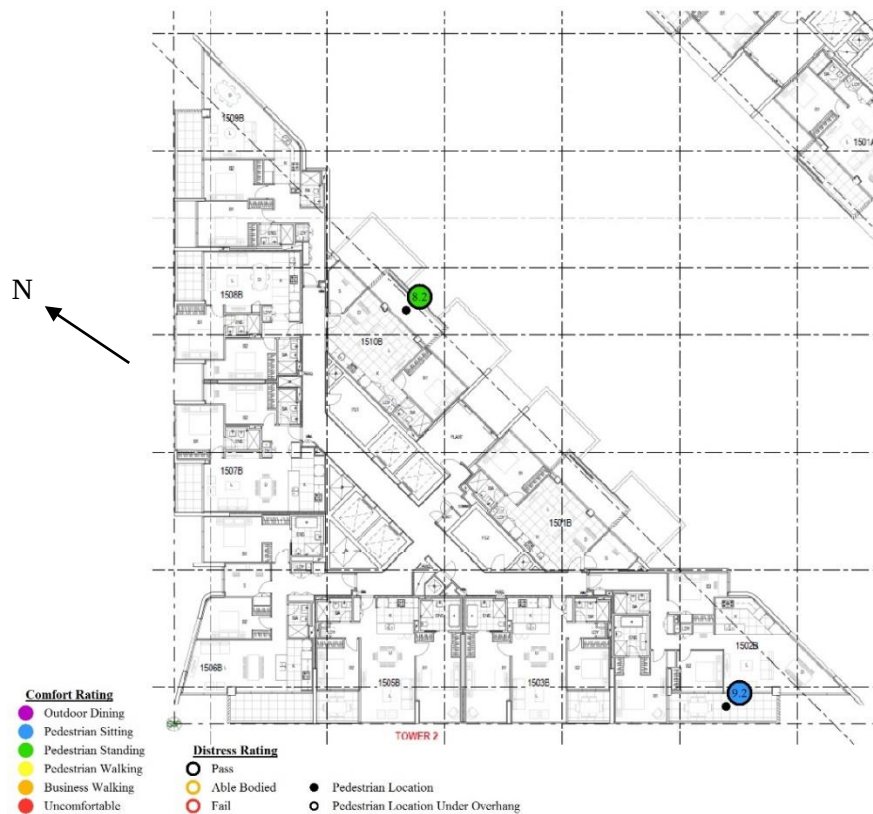
Figure 13: Level 31 balcony wind speed measurements – Configuration 2A
