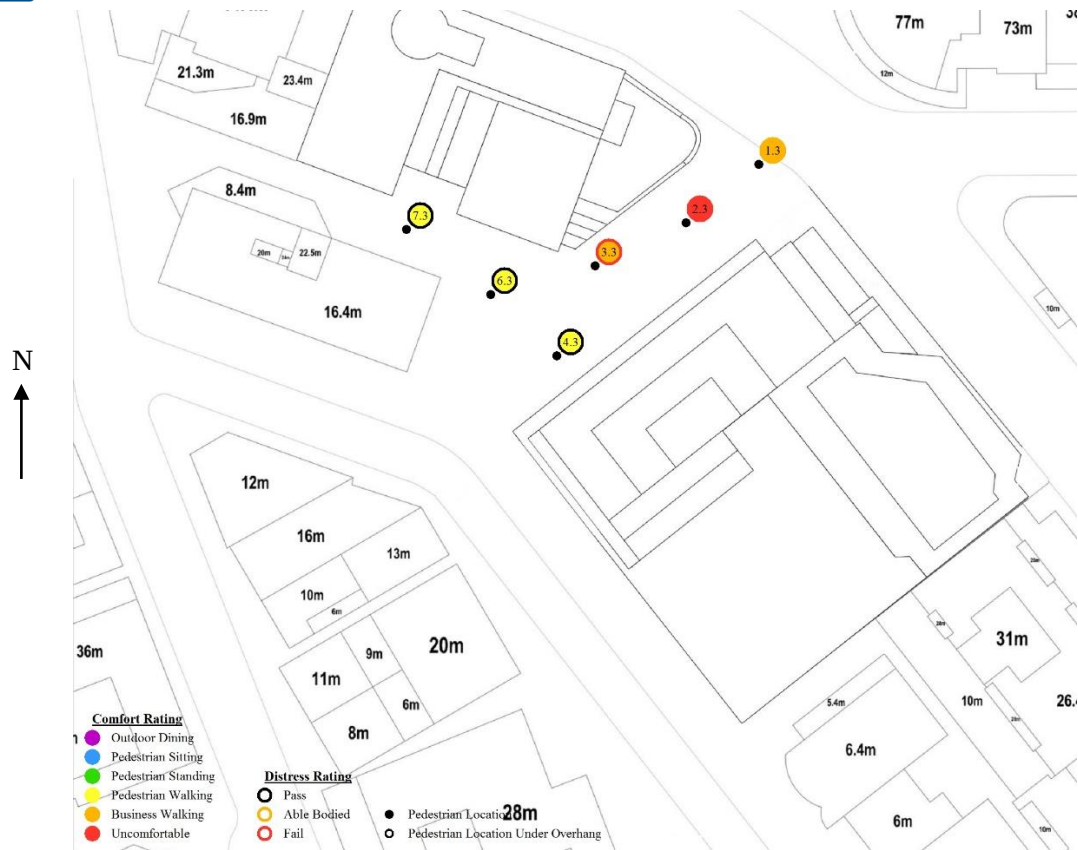
Figure 11: Pedestrian wind speed measurements – Configuration 3A, proposed 504 PH only
