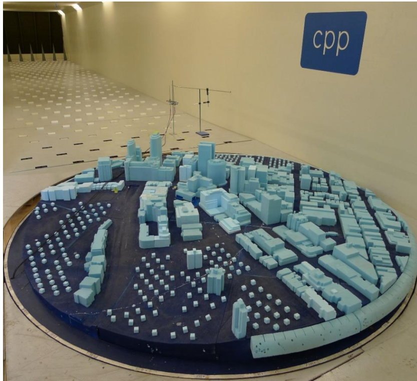
Figure 4: Photograph of the model in the CPP wind tunnel from the south – Configuration 1A
