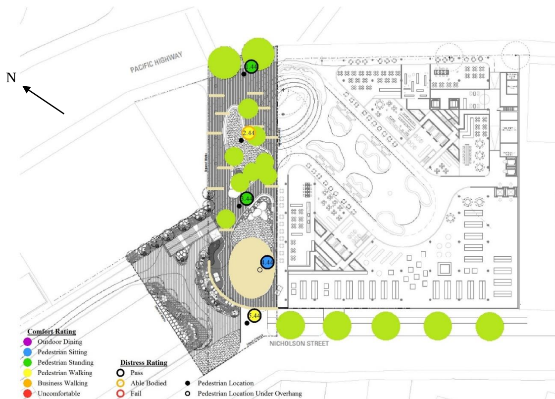
Figure 15: Pedestrian wind speed measurements – Configuration 4E
